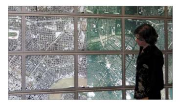
Researchers at the California Institute for Telecommunications and Information Technology developed the HIPerWall (Highly Interactive Parallelized Display Wall), the world's highest-resolution gridbased display for visualizing and manipulating massive data sets. Measuring over 200 square feet, the 50-panel wall brings to life terabyte-sized data sets, including biomedical images, climate datasets, and geological data.
